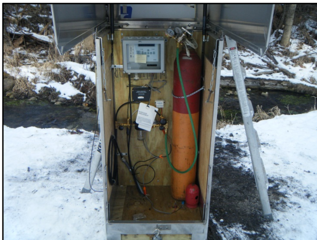
Nitrogen tank, pressure transducer, datalogger, and telemetry equipment inside the gaging station
